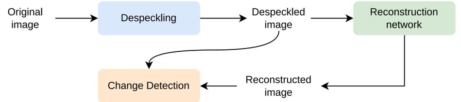
We adopt the anomaly detection methodology proposed in [3], which locates abnormal pixels by computing the deviation of a zone characteristics to the normal distribution. Instead of using the proposed AAE, we study an extension of the VAE family, called  $\beta$ -annealing VAE [2].
