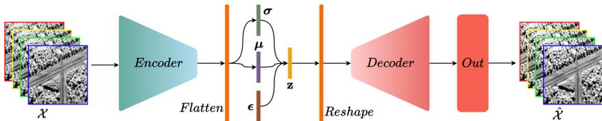
VAE architecture.  $\mathcal{X}$  and  $\hat{\mathcal{X}}$  denote respectively despeckled and reconstructed SAR images. To obtain  $\mathcal{X}$ , we apply MERLIN algorithm [1] on a Side Look Complex SAR image.
